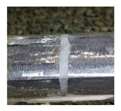
Belzona 1221 (Super E-Metal) is a two component emergency repair composite based on a ceramic steel reinforced polymer system. This fully machinable Belzona product can be used for the permanent bonding, repairing or rebuilding of metallic components.
